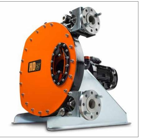
The peristaltic (hose) pump's ability to maintain excellent volumetric consistency and provide suction lift up to 9 meters (29.5 feet) makes it ideal for the 24/7 operating cycles that are common in oil-and-gas production.
