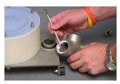
Draw the O-rings port outside [7] off the side housings [1]. Remove the inner O-rings [6] out of the ports [2].
