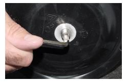
Screw out the set screws, shaft [13a].
