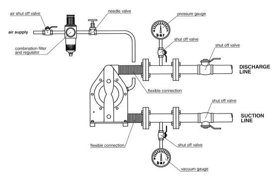
This illustration is a generic representation of a G Series air operated double-diaphragm pump.
