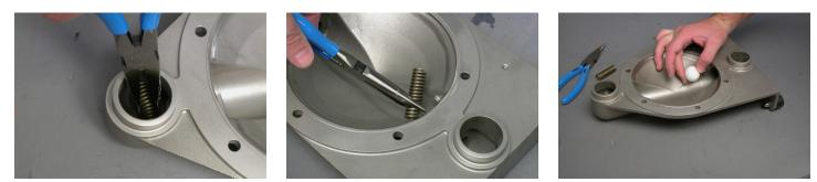
Remove the valve stops [3] and the ball valves [15] out of the side housings [1]. For the G125 and G200 the use of a screwdriver to remove the valve stops maybe is more convenient.
