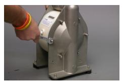
Loosen nuts of the housing bolts on one side of the pump.
