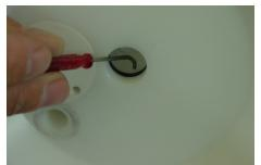
Remove both parts of the shaft piston rings [17] from their grooves carefully (do not damage the edges in the center block; a re-assembly of the same piston rings is impossible; they have to be replaced). Unscrew the muffler [20], the air inlet [18] and the air filter [19] out of the center block [16].
