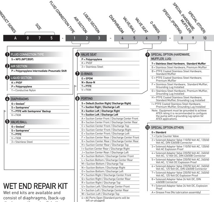
Wet end kits are available and consist of diaphragms, (back-up diaphragms if required), balls, seats and seat 0-Rings.
