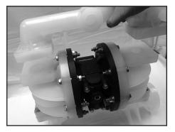
STEP 2 Remove the "Discharge Manifold".
