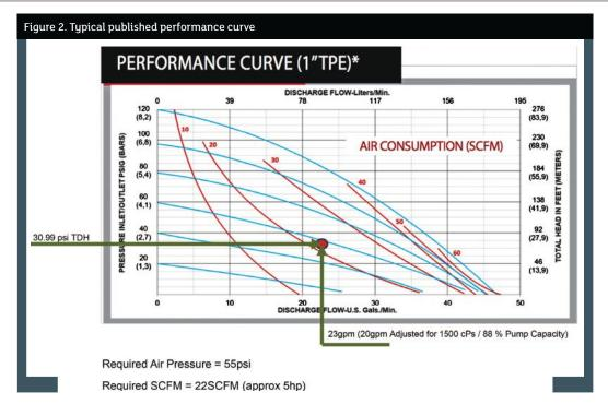
Viscosity and pipe diameter play a significant role in suction line loss and must be considered during evaluation. The system capabilities are limited by the pump's suction lift capabilities and air-inlet pressure.
