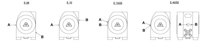
A = Air inlet for the pump, B = Air inlet for the pneumatic stroke counting system
