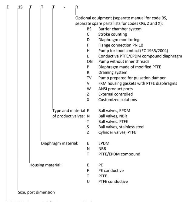
ALMATEC air-operated diaphragm pump, E-Series
