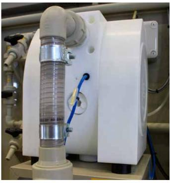
During their operation, injection-molded AODD Pumps can bounce, which can loosen pipework and increase the chances of a chemical leak. Almatec\* solid-body AODD Pumps are more stable during their operation, which leads to a higher level of product containment.
