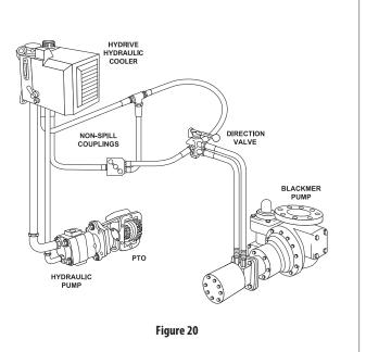
**Hydraulic driven units** are becoming more prevalent. They increase pump service life by eliminating the external loading on the pump shaft, which is inherent with a power take-off. They also provide, for more consistent speed control and "soft starting" of the pump.
