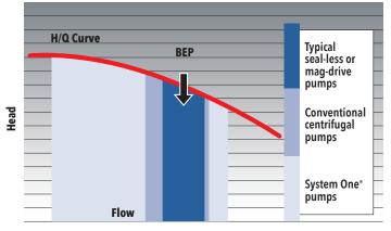
System One® Pumps resist vibration for a larger operational window off the BEP and greater reliability.
