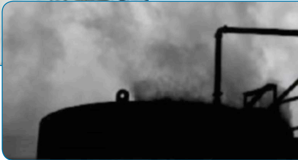
Photo taken at the same time with a FLIR® GasFinder infrared camera shows the vapors that are escaping
