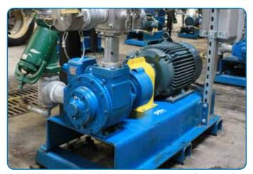
Blackmer® delivered the GX Series Sliding Vane Pumps to EMCO as part of an Engineered Package Solution that consisted of the pump, motor, coupling and coupling guard, all of which were attached to a baseplate for easy handling and installation.
