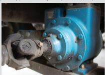
S.A. White Oil Company employs only Blackmer TXD Series Sliding Vane Pumps on its fleet of 25 fuel trucks to help deliver 80 million gallons of fuel a year.
