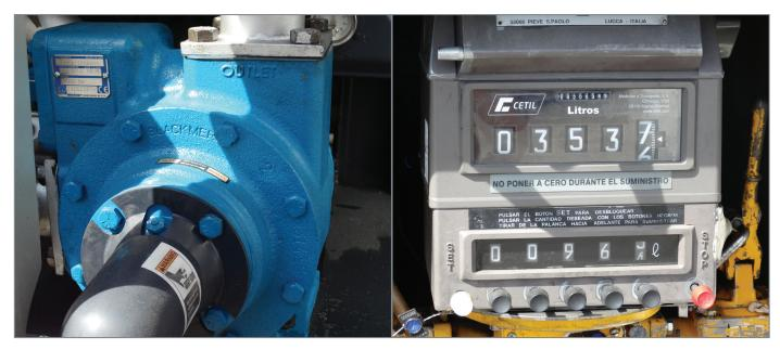
By combining Blackmer® TX Series Sliding Vane Pumps, left, with Cetil Dispensing Technology's metering equipment and systems, Reques e Hijos has optimized the performance of its truck-mounted fuel-delivery systems.
