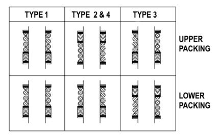
**SEAL ORIENTATION - DOUBLE SEAL COMPRESSORS**
