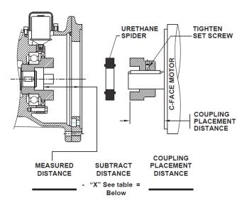
Jaw Style NEMA Motor Coupling Installation
