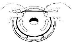
Figure 8 - Head O-Ring Installation
