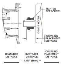
"M" Style NEMA Motor Coupling Installation
