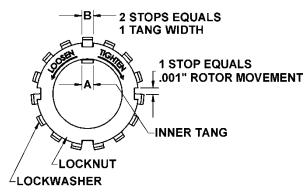
Figure 9 – Locknut Assembly
