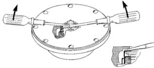
Figure 5 - Mechanical Seal Removal
