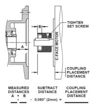
"J" Style NEMA Motor Coupling Installation
