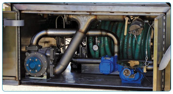
Transport companies are able to tap into the emerging Diesel Exhaust Fluid (DEF) market and delivery bulk quantities of DEF with the help of the new Blackmer line of STX3-DEF sliding vane pumps.
