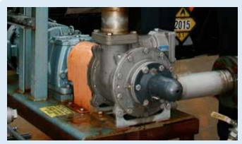
Blackmer® SNP Series Sliding Vane Pumps offer operational advantages for two seemingly unrelated industries-the manufacture of biodiesel and soap and detergents-with waste elements from the first able to be used to create end-products for the second.
