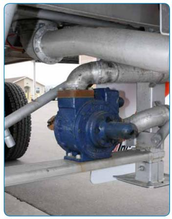
All Blackmer sliding vane pumps for biodiesel applications feature UL-listed and approved elastomer seals that allow for compatibility with all biodiesel blends, including B100.
