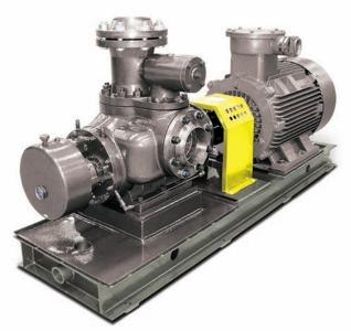
Blackmer S Series Twin Screw Pumps With Timing Gear (WTG) have been designed with external bearings and a timing-gear transmission, which produces double-suction, self-priming operation with no metal-to-metal contact between the pump's internal components. This design helps the pump achieve the highest flow rates of any rotary PD pump, even at varying backpressures and viscosity levels.
