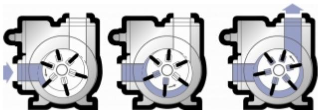
© Blackmer/Ebsray **The sliding vane pumping principle is perfect for autogas handling as it delivers smooth, consistent, non-pulsating flow, even at high differential pressures**
