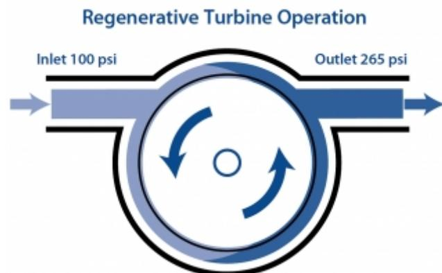
© Blackmer/Ebsray **The design of a regenerative turbine pump is unique and works on a different principle than positive displacement pumps. This design, however, allows the pump to operate cavitation-free at speeds up to 3,800 rpm and at high differential pressures with low flow rates, which makes it ideal for use in autogas-handling applications.**
