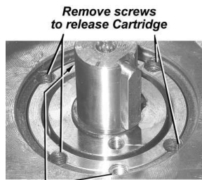
Insert screws to withdraw Cartridge Fig. 2
