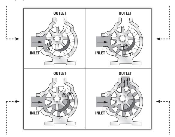
As the rotor continues to turn, the liquid is forced past the crescent-shaped area and moves toward the discharge port.
