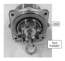
Tool Inserted in Rotor Assembly
