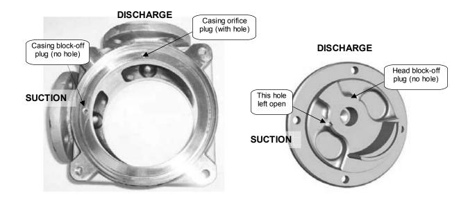
Special Cooling Circuit Plugs in Correct Positions
