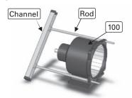
Assemble Rods and Channel
