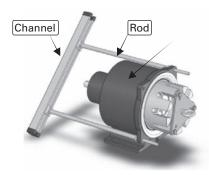
Attach Rods and Channel
