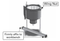
Outer Drive Assembly Mounted to Tool
