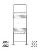
IDLER BUSHING PROTRUSION (E1-133 and E1-222 Models)
