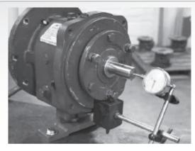
FIGURE 20 BEARING END PLAY CHECK
