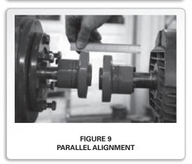
With coupling hubs stationary, lay straight edge flat against rim of coupling hub to determine vertical and horizontal alignment offsets. Adjust and/or shim equipment until the straight edge lies flat against both hub rims, vertical and horizontal.
