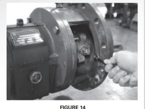
FIGURE 14 STUFFING BOX COVER REMOVAL
