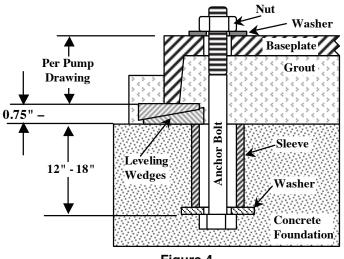
Figure 4 Typical Anchor Bolt (Sleeve Type)
