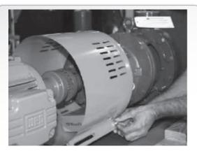
FIGURE A-3 COUPLING GUARD BARREL
