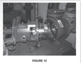
FIGURE 12 BACK PULL-OUT REMOVAL
