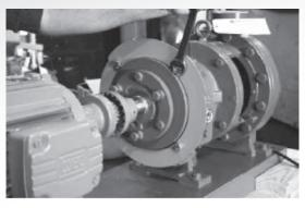
FIGURE A-2 COUPLING GUARD END PLATE
