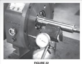
FIGURE 22 FRAME FACE RUNOUT CHECK
