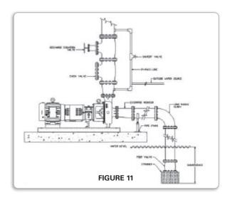
See illustration at left. Note vent location above pump discharge nozzle.
