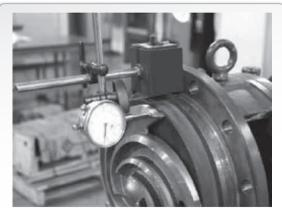
FIGURE 25 IMPELLER RUNOUT CHECK
