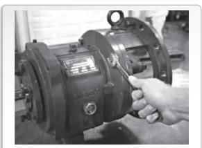
FIGURE 15 ADAPTER REMOVAL Frame adapters are used on M, L and XL group pumps. They are not used on 6" S group pumps and ring adapters are on 8" S group pumps.
