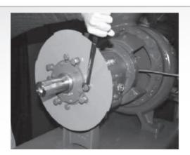
FIGURE A-2 811XL COUPLING GUARD END PLATE
