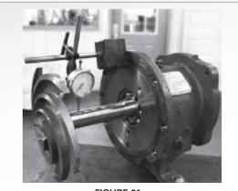
FIGURE 21 SHAFT RUNOUT CHECK
