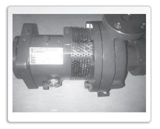
When ordered, the pump will be shipped with the seal guard installed. The seal guard is supplied with captive fasteners to secure the guard in place.
