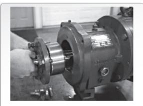
FIGURE 16 SHAFT/BEARING HOUSING REMOVAL
