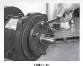
FIGURE 26 PRELIMINARY IMPELLER ADJUSTMENT
