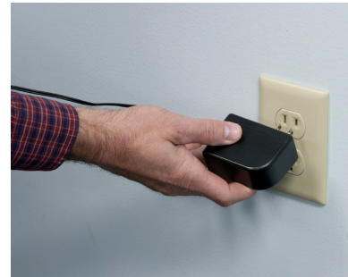
Step 1 - Plug wall transformer into AC outlet
