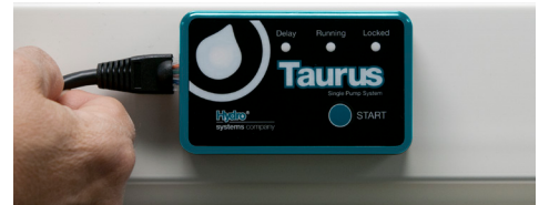
Step 4 - Connect Cat 5 cable to remote
