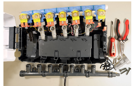
9) Lift manifold to provide clearance
