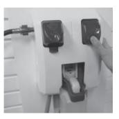
14. To operate button fill units, depress button to dispense product, release button to stop flow. IF YOU WISH TO LOCK THE BUTTON IN THE "ON" POSITION: Depress button and slide button lock up, TO UNLOCK, DEPRESS BUTTON AND RELEASE.
