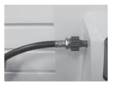
11. Connect water supply hose of at least 3/8" ID to water inlet swivel. Min. 25 psi pressure is required for proper operation, Max. pressure 85 psi and 120°F Max. water temperature. Connect opposite end of hose to water supply. Turn water supply on.
