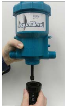
Step 1. Unscrew and remove lower end from assembly.
