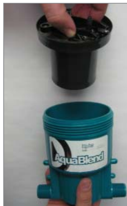
Step 5. Remove motor piston from pump body.
