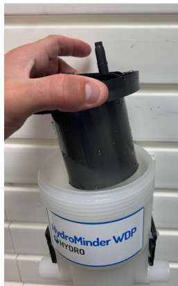
Step 5. Remove motor piston from pump body.
