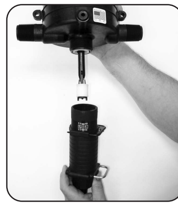
Step 8. Screw LOWER END CYLINDER ASSEMBLY onto body. Ensure #16 gasket is seated on the top of cylinder assembly.
