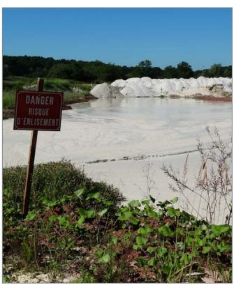
The highly viscous nature of the wastewater at the Sables et Mineraux mine is attested to by the warning sign at the facility's retention area: "Danger: Risk of getting bogged down" it reads, an admonition to avoid stepping into the quicksand-like substance.
