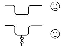
If installation is heated, it must be designed so that fluid dilatation can evacuate through piping. Therefore fluid contained in piping must be heated before fluid contained in the pump. Also check that a heated pump is not isolated by closed valves.
