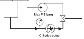
We recommend limiting the rotation speed of the C Series pump.
