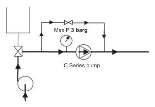
It is preferable not to run the C Series pump during CIP, although low speed (< 100 rpm) is acceptable by alternating start/stop operation.
