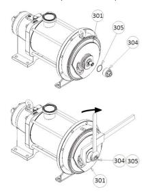
It is important to keep a good grip on the piston; its rotation could lead to deterioration of the bellows.
