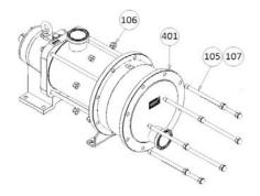
• Remove the front cover 401. If the discharge piping is mounted in a rigid manner, pivot the bottom 401 so as to free the connection.
