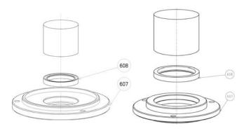
• If the seal face is marked, change the ring 507. Break the ring with a chisel then fit a new ring after heating it at 90°C (in an oil bath or at HF).
