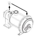
Screw the lifting hook in the tapped hole of the cylinder, provided for this purpose and tighten the screw in the location of the lifting ring.
