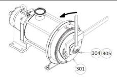
To make handling of the cylinder/piston unit easier, move the lifting ring from the transmission body to the cylinder.
