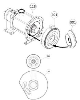
Place thread locking adhesive (Loctite® 243\* or equivalent) on the thread of the transmission hub 596.
