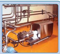
Mouvex C-Series C18i Eccentric Disc Pump.
