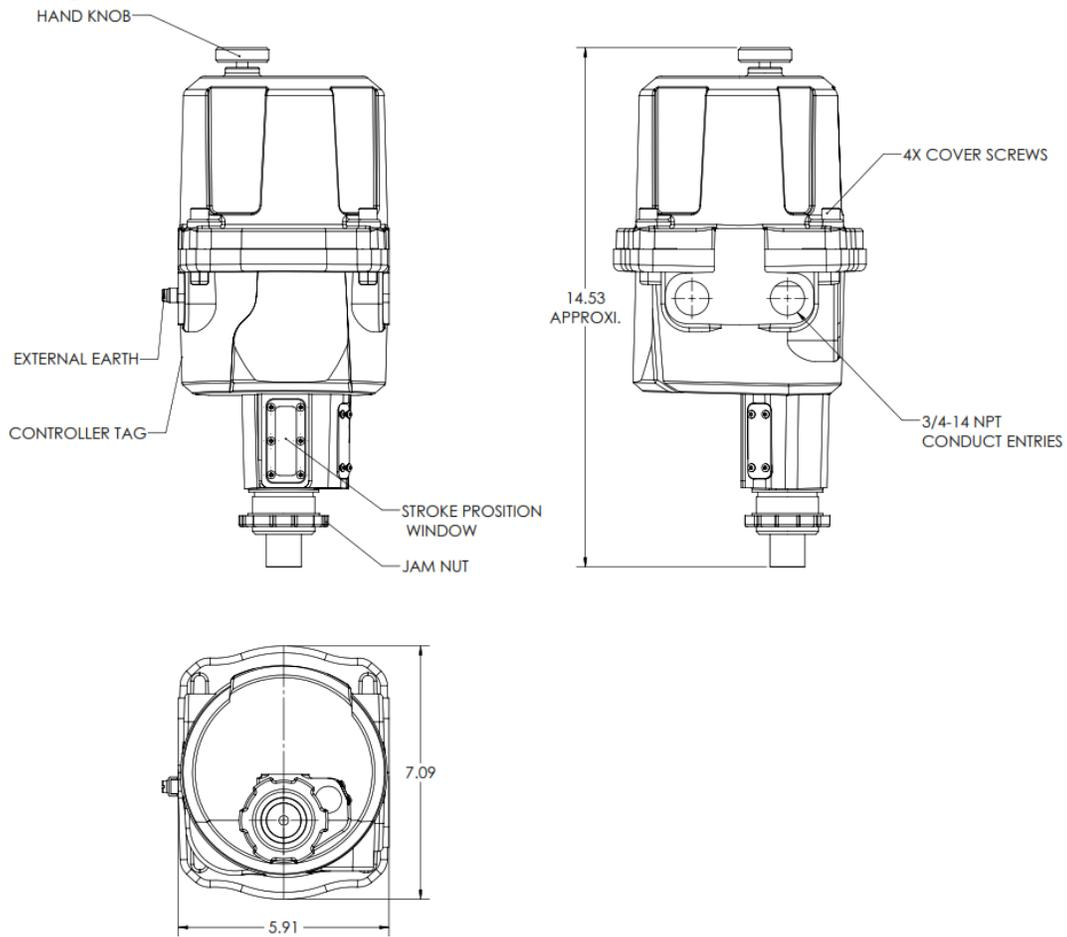
**Handwheel Operation** The handwheel is located on the top cover. Push and hold the handwheel down and rotate to extend/retract or rotate the actuator output drive. Verify direction of output shaft rotation for clockwise operation of the handwheel. Stroke position can be found at the local display window
