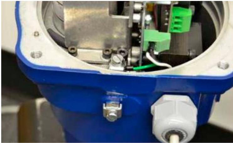
A lug is cast adjacent to the conduit entries for attachment of an external protective Earth (Ground) cable. An internal earth terminal is also provided. Consult local and certifying agency codes to determine which earth connectors is to be used.
