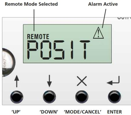
Four push button switches are located on the main PCB below its LCD Display and are used to view and change the actuator configuration parameters.
