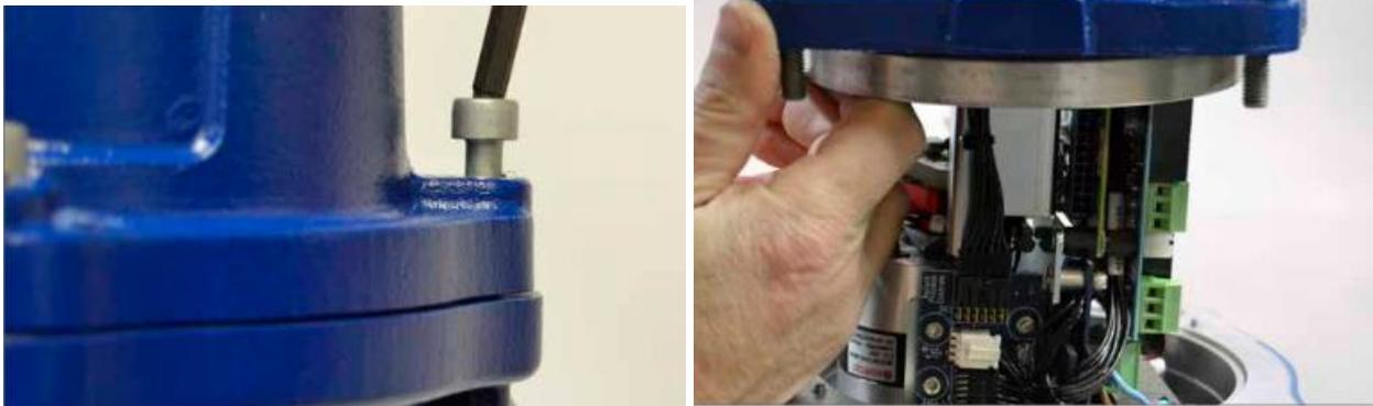
Using a 6 mm Allen key loosen the captive fixings securing the terminal compartment cover. Do not attempt to lever off the cover with a screwdriver as this will damage the o-ring seal and may damage the flamepath on a certified unit.
