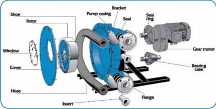
The simple design of the Abaque Series Peristaltic (Hose) Pumps features a seal-free design that eliminates leaks and product contamination, which enables them to handle the paint and coatings industry's toughest pumping applications.
