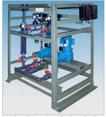
Mechanically actuated diaphragm metering pumps offer excellent suction lift capabilities, ease of operation and start-up, and the ability to handle liquids that off gas, which makes them an ideal option for chemical-handling applications at wastewater-treatment facilities.
