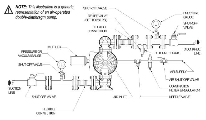
**NOTE:** In the event of a power failure, the shut-off valve should be closed, if restarting of the pump is not desirable once power is regained.
