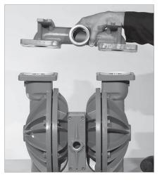
Step 6 Remove the inlet manifold to expose the valve ball, valve seat and plug.
