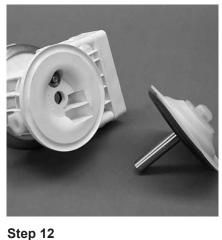
To remove the remaining diaphragm assembly from the shaft, secure shaft with soft jaws (a vise fitted with plywood or other suitable material) to ensure shaft is not nicked, scratched, or gouged. Using an adjustable wrench, remove diaphragm assembly from shaft. Inspect all parts for wear and replace with genuine Wilden parts if necessary.
