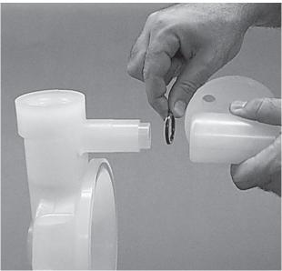
**Step 10**Remove tee section from liquid chamber and inspect O-rings for signs of wear. Replace worn parts with genuine Wilden parts for reliable performance.
