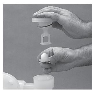
**Step 3**Remove the top liquid retainer to expose the valve balls, valve seats and valve seat O-rings.
