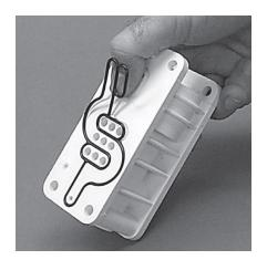
Lift away air valve assembly and remove air valve gasket for inspection. Replace if necessary.
