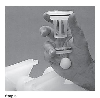
Remove the bottom liquid retainer and retainer O-rings, discharge valve balls, seats and valve seat O-rings from the liquid chamber and inspect for nicks, gouges, chemical attack or abrasive wear. Replace worn parts with genuine Wilden parts for reliable performance.
