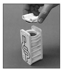
Loosen the air valve bolts utilizing 3/16"
