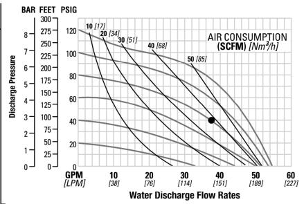
Example: To pump 140 lpm (37 gpm) against a discharge pressure head of 2.8 bar (40 psig) requires 5.5 bar (80 psig) and 60 Nm3/h (38 scfm) air consumption.
