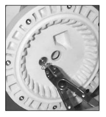
Remove pilot spool sleeve retaining snap
