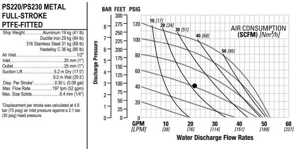
Example: To pump 83.3 lpm (22 gpm) against a discharge head of 2.8 bar (40 psig) requires 4.1 bar (60 psig) and 36 Nm<sup>3</sup>/h (23 scfm) air consumption.
