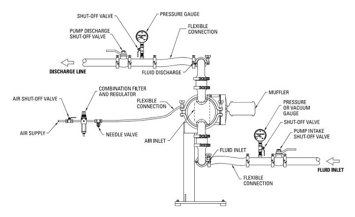
NOTE: In the event of a power failure, close the shutoff valve if you do not want the pump to restart when the power returns.
