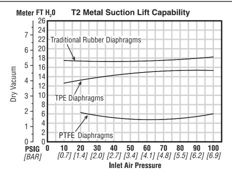
Suction lift curves are calibrated for pumps operating at 305 m (1,000') above sea level. This chart is meant to be a guide only. There are many variables which can affect your pump's operating characteristics. The number of intake
