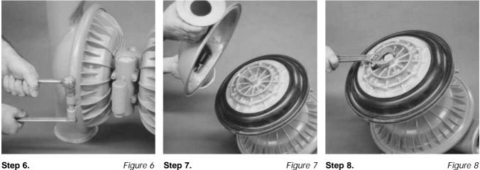
With 3/4" socket and 3/4" box wrench, remove one set of large clamp bands that attach liquid chamber to center section assembly.
