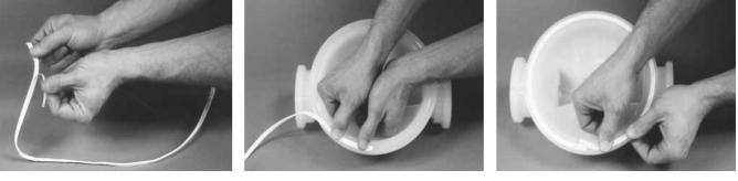
Figure 1 Step 2. Gently remove the adhesive covering Starting at any point, place the PTFE from the back of the PTFE tape. Ensure tape in the center of the diaphragm bead that the adhesive strip remains attached groove on the liquid chamber and press lightly on the tape to ensure that the adhesive holds it in place during assembly. Do not stretch the tape during placement in center of diaphragm bead groove.
