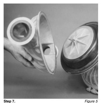
Lift liquid chamber away from center section to expose diaphragm and outer piston. (*Figure 7*)
