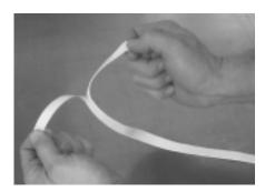
Step 1.Figure 1Gently remove the adhesive covering<br/>from the back of the Teflon® tape. Ensure<br/>that the adhesive strip remains attached<br/>to the Teflon® tape and is not removed<br/>with the adhesive covering.
