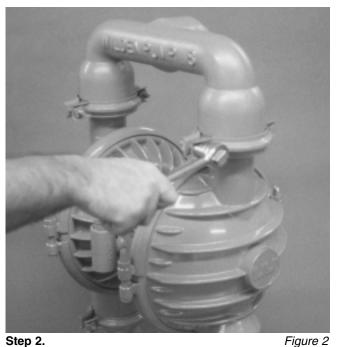
Utilizing the 13 mm (1/2") box wrench, remove the two small clamp bands that fasten the discharge manifold to the liquid chambers. (Figure 2)
