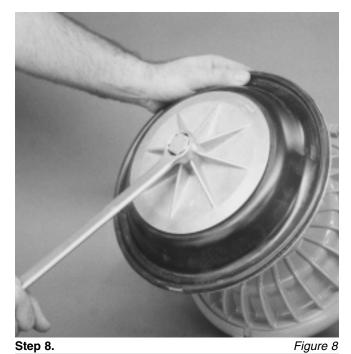
Using a 25 mm (1") box wrench, adjustable wrench, or by rotating the diaphragm by hand, remove the diaphragm assembly.
