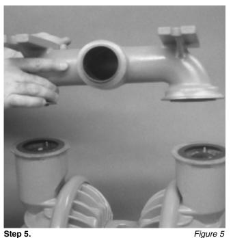
Lift the intake manifold away to expose the valve balls and seats. Inspect intake valve ball cage for excessive wear or damage. Remove the intake valve balls, seats and o-rings from the discharge manifold and inspect for nicks, gouges, chemical attack or abrasive wear. Replace worn parts with genuine Wilden parts for reliable performance. Teflon® o-rings should be replaced when reassembled. (*Figure 5*)
