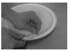
Step 3.Figure 3The end of the tape should overlap<br/>approximately 13 mm ( $\frac{1}{2}$ ") (Figure 3).Proceed to install the Teflon® tape on the<br/>remaining diaphragm.
