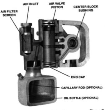
NOTE: Air valve available with or Figure B without oil bottle and capillary rod.
