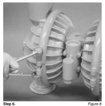
With 14 mm (%<sup>6</sup>") socket and 17 mm ( $^{1}/_{16}$ ") box wrench, remove one set of large clamp bands that attach liquid chamber to center section assembly. (*Figure 6*)
