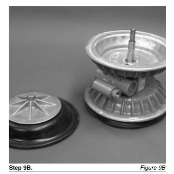
2) The outer piston, diaphragm, and inner piston separate from the shaft which remains connected to the opposite side diaphragm assembly (*Figure 9B*). Repeat disassembly instructions for opposite liquid chamber. Inspect diaphragm assembly and shaft for signs of wear or chemical attack. Replace all worn parts with genuine Wilden parts for reliable performance.
