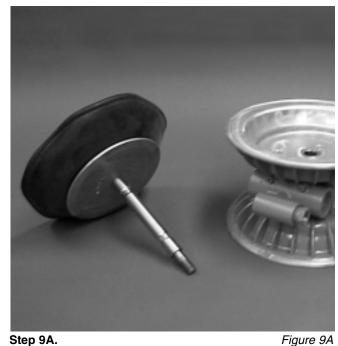
**NOTE:** Due to varying torque values, one of the following two conditions may occur: 1) The outer piston, diaphragm and inner piston remain attached to the shaft and the entire assembly can be removed from the center section. (*Figure 9A*)
