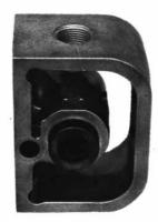
P/N 08-3300-07 Bronze Bushing can be pressed into a stainless steel or cast iron center section. (See *Figure F*). When installing a new bushing, four bleeder holes which allow the pump to exhaust air must be drilled. (See *Figure G*).
