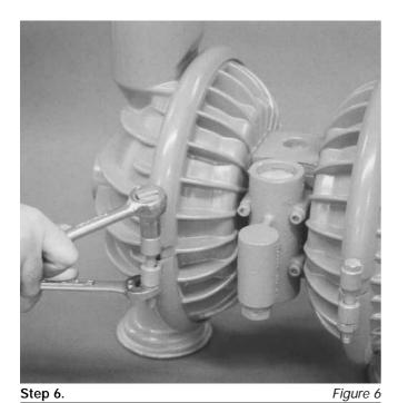
With 14 mm (9/16") socket and 17 mm (11/16") box wrench, remove one set of large clamp bands that attach liquid chamber to center section assembly.
