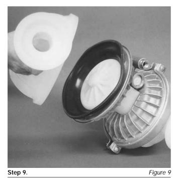
Lift liquid chamber away from center section expose diaphragm and outer piston.
