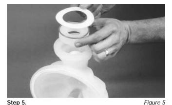
Install the valve ball, valve seat and o-ring.
