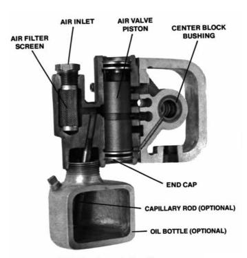
NOTE: Air valve available with or without oil bottle and capillary rod.
