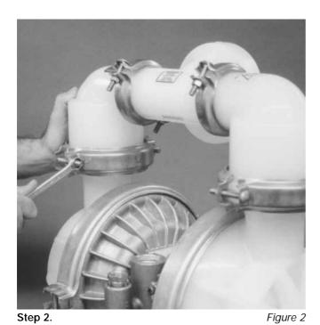
Utilizing a 13 mm (1/2") wrench, remove the two small clamp bands that fasten the discharge manifold to the liquid chambers.
