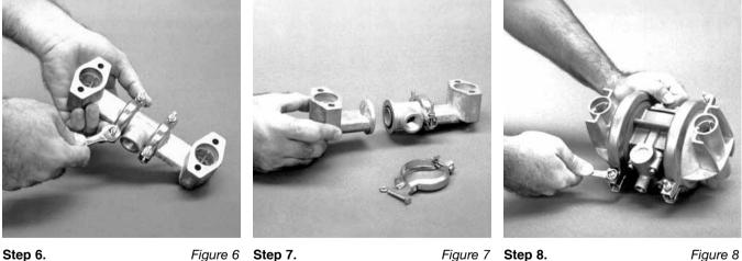
Normally the inlet and discharge manifold should not be disassembled during regular pump maintenance. Should this be necessary completely remove and disassemble manifold clamp bands.
