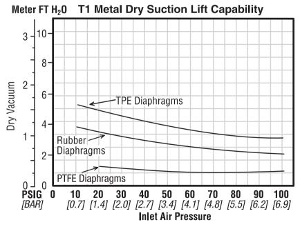
These vacuum numbers will double when a small amount of back pressure is placed on the discharge.
