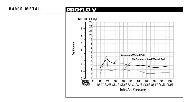
Suction lift curves are calibrated for pumps operating at 305 m (1,000') above sea level. This chart is meant to be a guide only. There are many variables which can affect your pump's operating characteristics. The number of intake and discharge elbows, viscosity of pumping fluid, elevation (atmospheric pressure) and pipe friction loss all affect the amount of suction lift your pump will attain.
