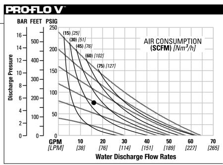
Flow rates indicated on chart were determined by pumping water. For optimum life and performance, pumps should be specified so that daily operation parameters will fall in the center of the pump performance curve. Air inlet pressure values are 50% of discharge pressure values shown on Y axis.
