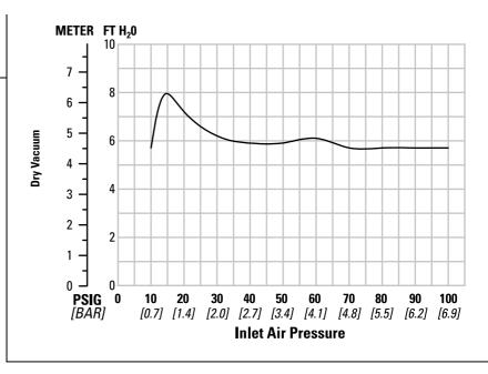
Suction lift curves are calibrated for pumps operating at 305 m (1,000') above sea level. This chart is meant to be a guide only. There are many variables which can affect your pump's operating characteristics. The number of intake and discharge elbows, viscosity of pumping fluid, elevation (atmospheric pressure) and pipe friction loss all affect the amount of suction lift your pump will attain.
