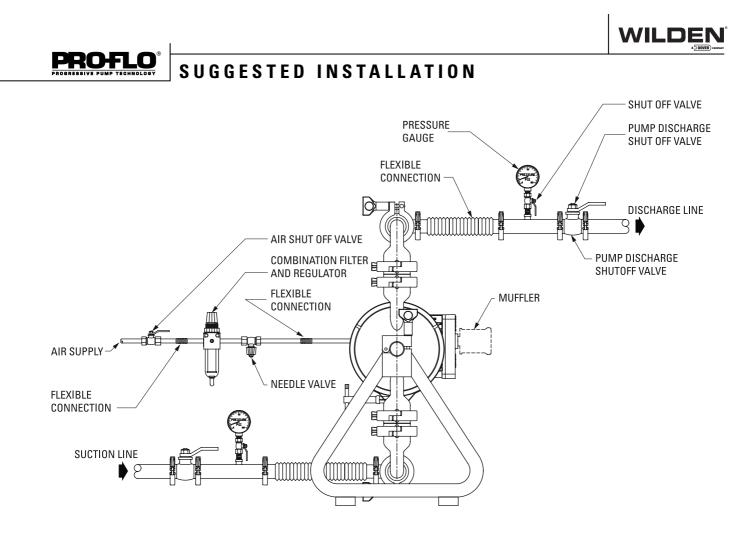
**NOTE**: In the event of a power failure, the shut off valve should be closed, if restarting of the pump is not desirable once power is regained.
