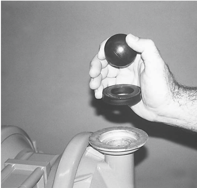
Step 4. Figure 4 Remove the discharge valve balls and seats ( Figure 4 ) from the liquid chambers and inspect for nicks, chemical attack or abrasive wear. Replace worn parts with genuine Wilden parts for reliable performance.
