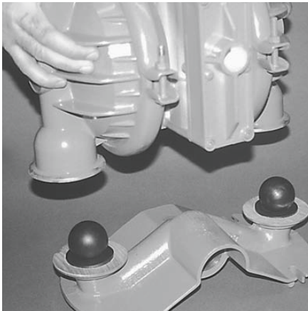
Step 6. Figure 6 Lift liquid chambers and center section from intake manifold to expose intake valve balls and seats. Inspect ball cage area of liquid chamber for excessive wear or damage. ( Figure 6 )
