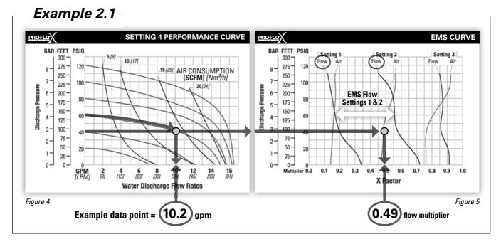
This is an example showing how to determine the inlet air pressure and the EMS setting for your Pro-Flo  $X^{\text{TM}}$  pump to optimize the pump for a specific application. For this example we will be using an application requirement of 18.9 lpm (5 gpm) flow rate against 2.8 bar (40 psig) discharge pressure. This example will illustrate how to calculate the air consumption that could be expected at this operational point.
