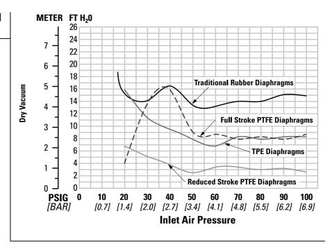
Suction lift curves are calibrated for pumps operating at 1,000' (305 m) above sea level. This chart is meant to be a guide only. There are many variables which can affect your pump's operating characteristics. The number of
