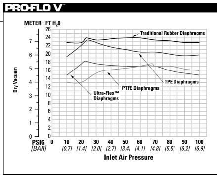
Suction lift curves are calibrated for pumps operating at 305 m (1,000') above sea level. This chart is meant to be a guide only. There are many variables which can affect your pump's operating characteristics. The number of intake and discharge elbows, viscosity of pumping fluid, elevation (atmospheric pressure) and pipe friction loss all affect the amount of suction lift your pump will attain.
